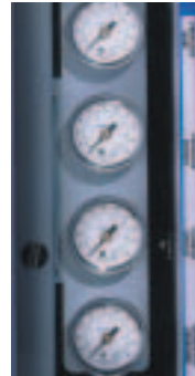
Internal gauges allow you to monitor membrane and filter pressures
